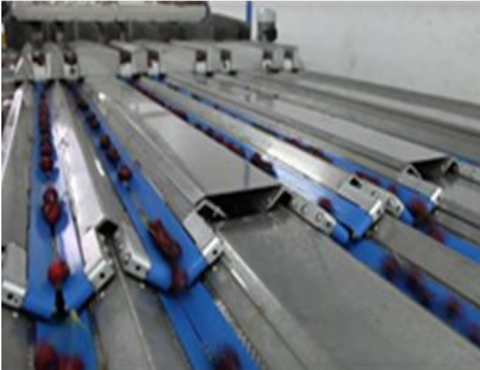
V-ledge belts in washing and sorting units for fruits
