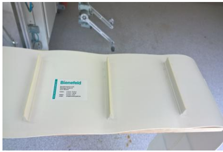
Conveyor belt with T-bars
