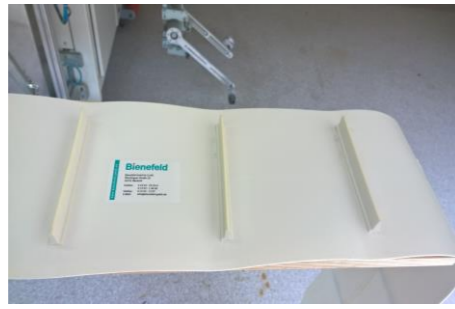
Conveyor belt with T-bars
