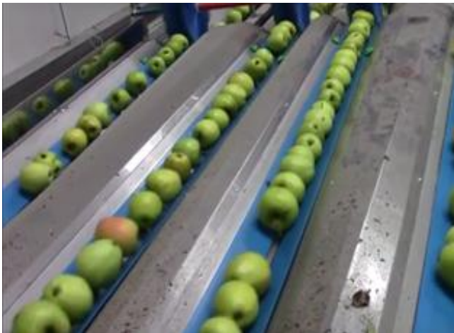
Profile belts with longitudinal grooves for transporting cherries and apples from the washing unit to sizing.
