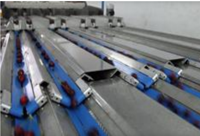
Profile belts with longitudinal grooves for transporting cherries and apples from the washing unit to sizing.
