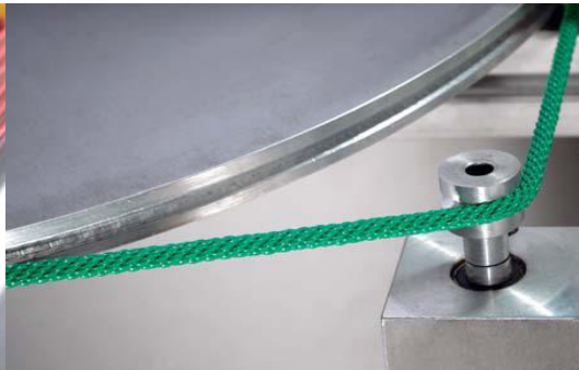
Endless turned round belt PU green, suitable for exceptional transmissions
