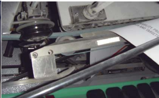
2 mm polyester round belt in a folding machine for paper
