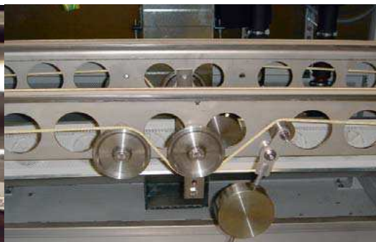
Endless turned round belt made of Kevlar in a transport line for cover frames
