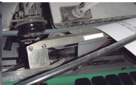
2 mm polyester round belt in a folding machine for paper
