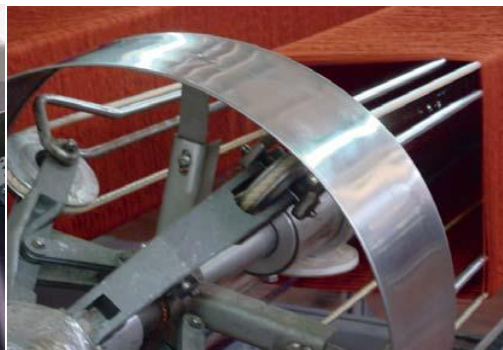
NOMEX-PTFE high bulk belts in a textile finishing installation
