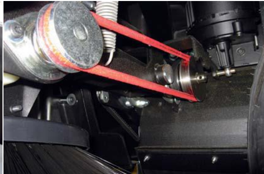
Lateral broom drive of a power sweeper
