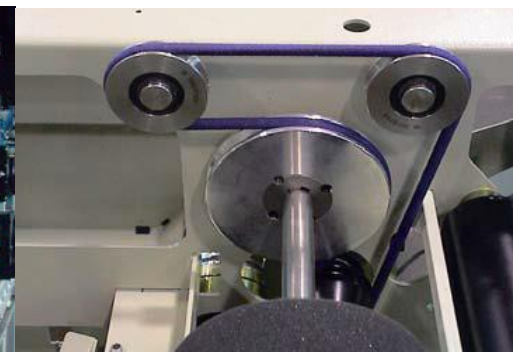
Roller drive in a plaiting machine
