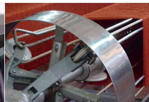
NOMEX-PTFE high bulk belts in a textile finishing installation
