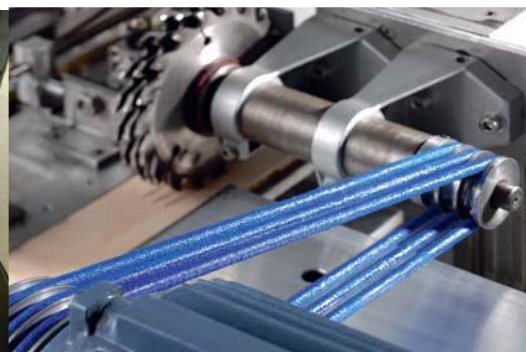
Endless elastic round belt, PU blue in a woodworking machine
